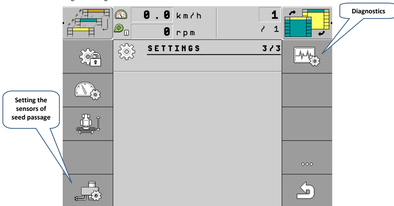
Picture 22 – Setting the sowing sensors
