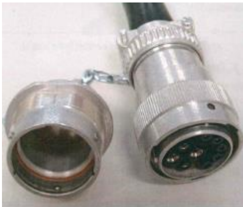
Picture. 4 - Connection socket on the tractor
