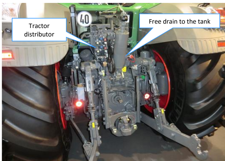
Picture. 6 – Position of quick couplings in the tractor
