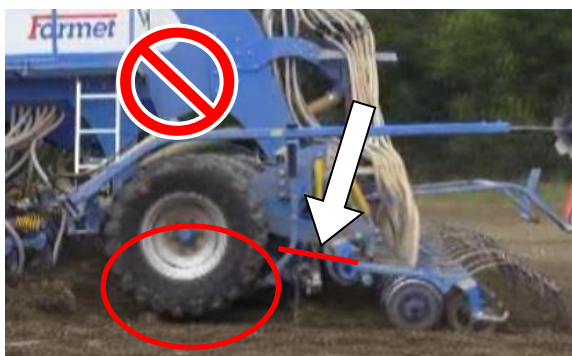
Picture 58 – Location of the sowing body pressure gauge
