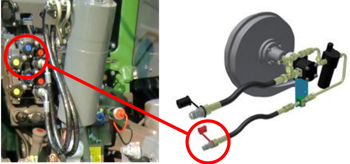
Picture 24.4 – Pressure hose connection
