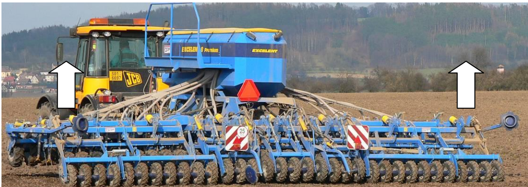
Picture 17 – Lifting the side sections of the rear rolls
